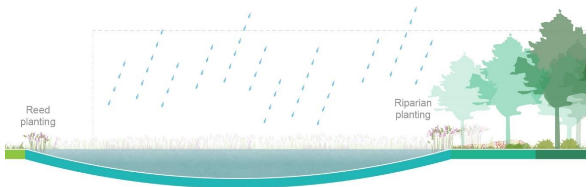
Plate 4-27 Example of attenuation pond function
