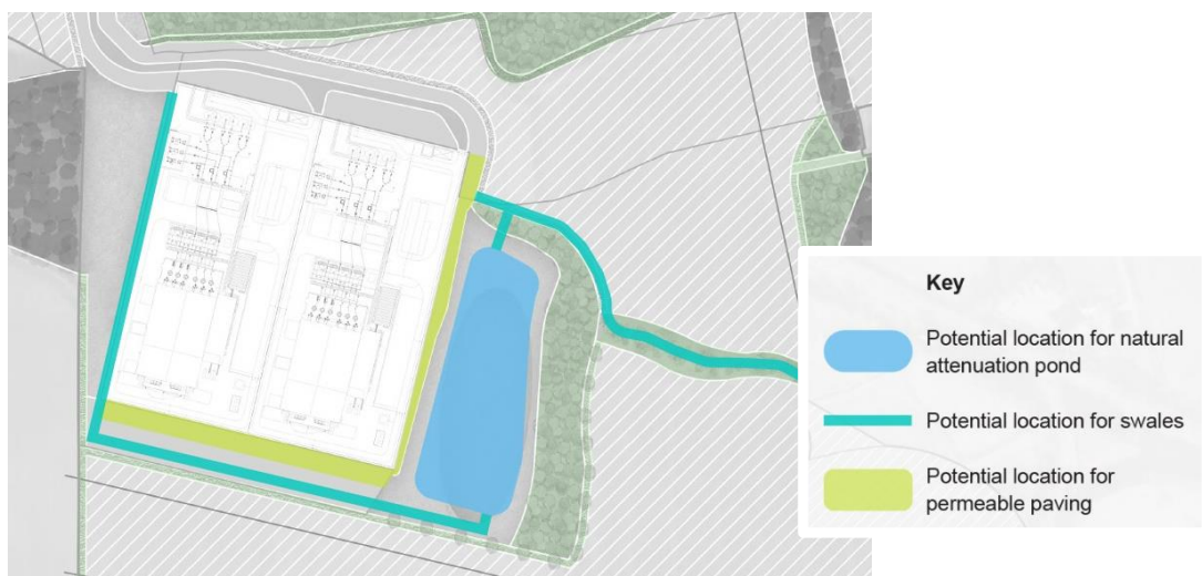
Plate 4-28 Example of swales around the Onshore Converter Stations
